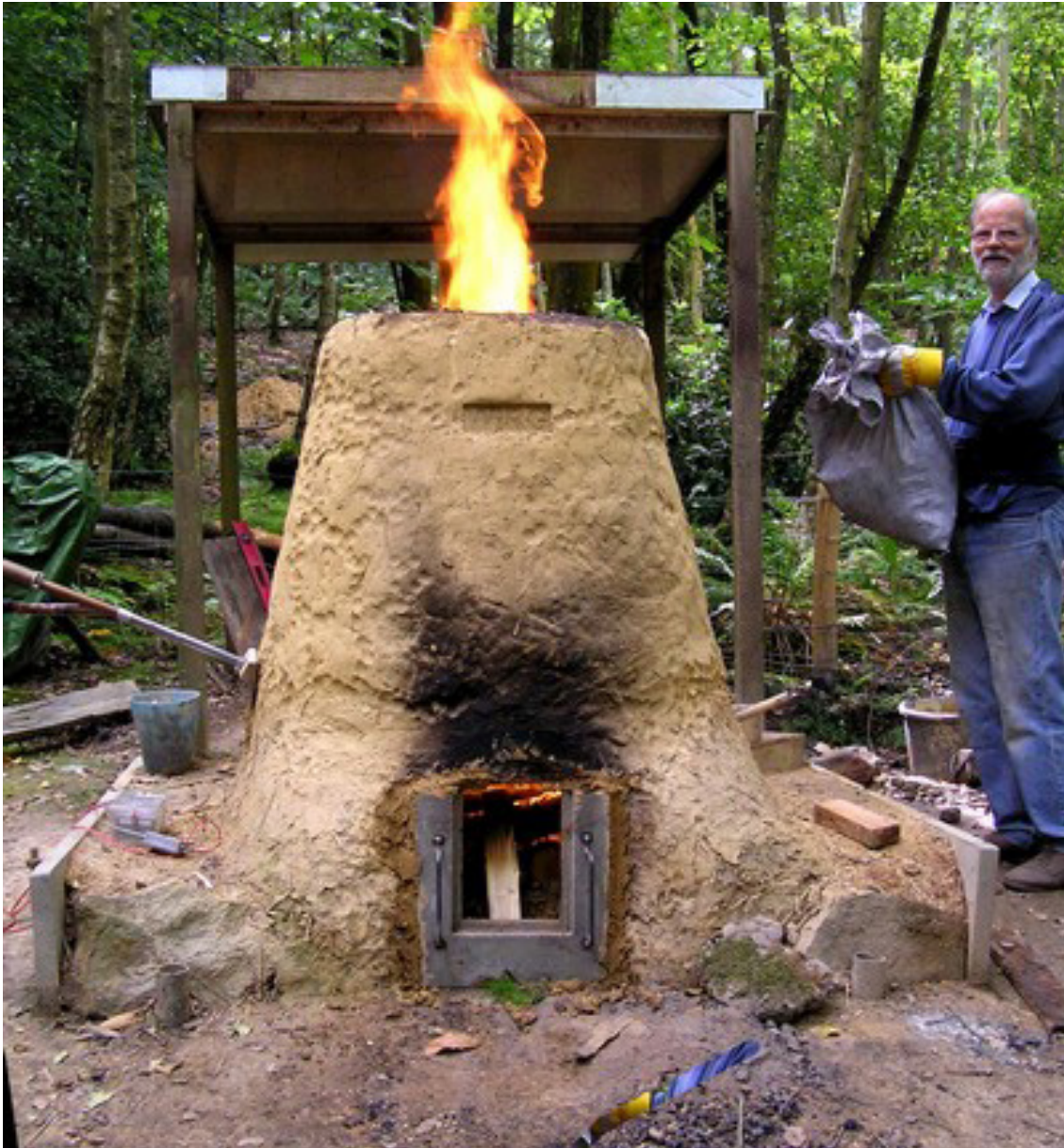
Experimental bloomery made by the Wealden Iron Research Group in October 2012. Here the furnace is being preheated to 800°C with charcoal. © WIRG
